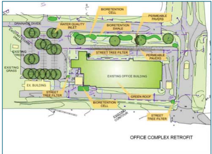
Green Infrastructure retrofit design at the Anacostia Annex of the Washington Navy Yard. (Department of Defense)
